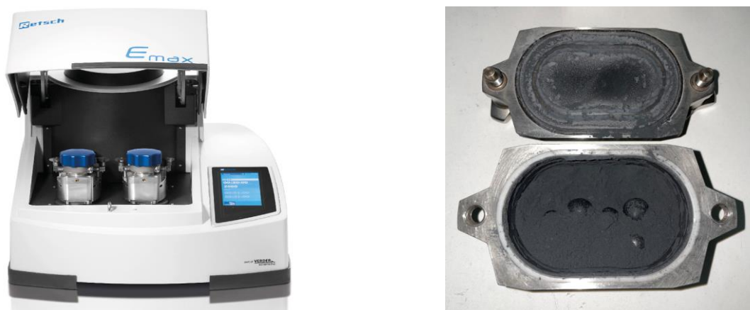
Figure 3 - Retsch E max high-speed ball mill, grinding cup and grinding balls
