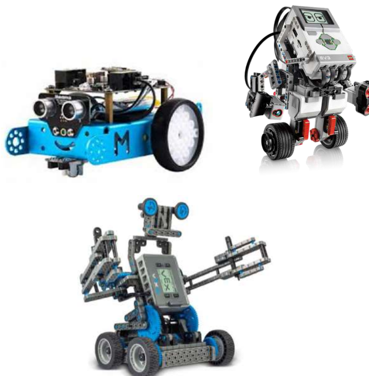
Figure 1. The types of robots - MBOT (Arduino) LEGO, MINDSTORMS EV3 VEX IQ
