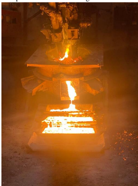
Figure 5 - Metal and slag discharge from the furnace
